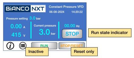
When the switch is OFF (Open Circuit) the Drive enters a no-run state and the run state indicator on the screen will display STOP.
