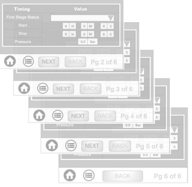
Once programming is complete, the 1<sup>st</sup> page of the timing group shows how many Stages are active AND which Mode they are set to.
