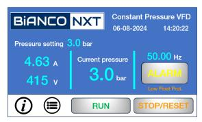
When the float switch falls to its OFF position, after the Pressure Group - Parameter #17, Water Shortage Delay Time has elapsed a message will appear on the screen "Low Float Prot".
