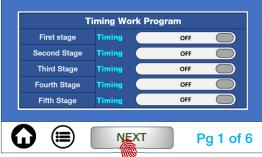
**Timing Work:** the controller will ONLY operate at the times and pressure(s) set at each stage
